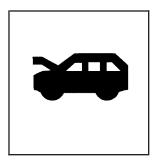
1. Pull the handle with this symbol on it. It is located under the instrument panel on the driver's side of the vehicle.
